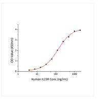
Immobilized Human IL-12B&IL-23A at 5 $\mu$ g/mL (100  $\mu$ L/well) can bind Human IL23R with a linear range of 4-135 ng/mL.
